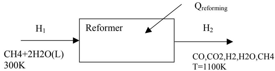
Using Equil one can calculate the mole fractions of the final stage and enthalpies of the initial and final stages. In the "Gas Chemistry input" (chem.inp) file in Equil, you need to specify CO, CO<sub>2</sub>, H<sub>2</sub>, H<sub>2</sub>O and CH<sub>4</sub>. Also, you need to supply "Surface chemistry input" for H<sub>2</sub>O in liquid form.<sup>1</sup> An example of input files is as follow:
