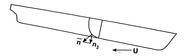
Here, for positive pitch, there is an upward (positive z) component of velocity equal to  $-U\zeta_5\,e^{i\omega t}$ . This has a component normal to the hull surface of  $-U\zeta_5 e^{i\omega t}n_3.$
