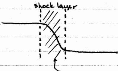
large viscous stresses + heat transfer } (due to large gradients in velocity + temp.)
