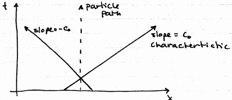
For nonlinear waves,  $u+c \neq \text{const} \therefore$  characteristics are no longer straight lines
