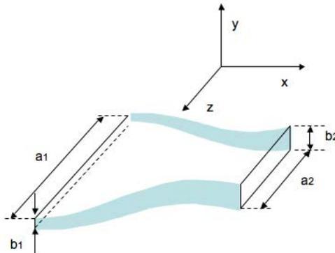
A steady, inviscid, incompressible flow experiences a change of cross sections between stations (1) and (2), as shown. At station (1), the velocity distribution is
