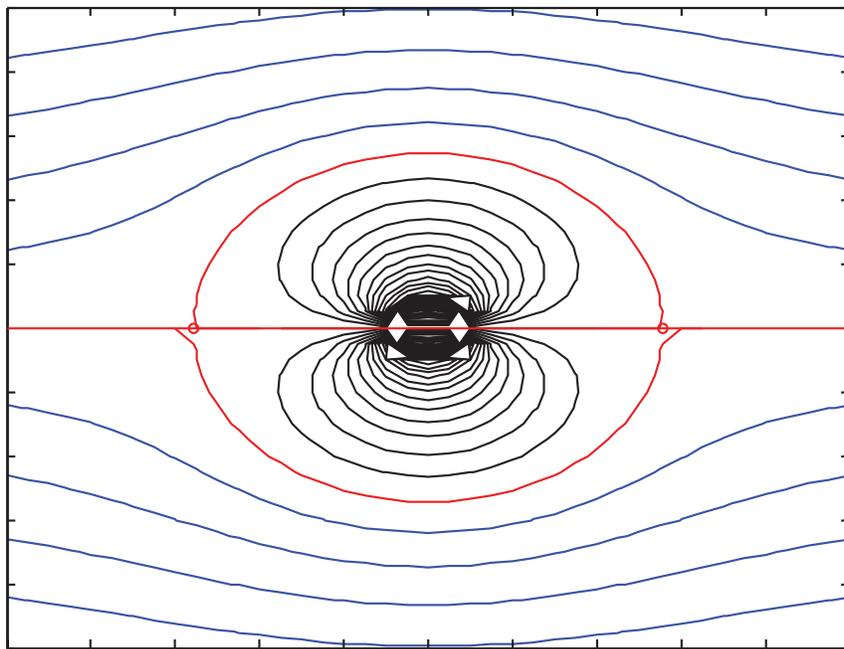
Figure 1: MATLAB<sup>®</sup> plot of streamlines for a Rankine oval.
