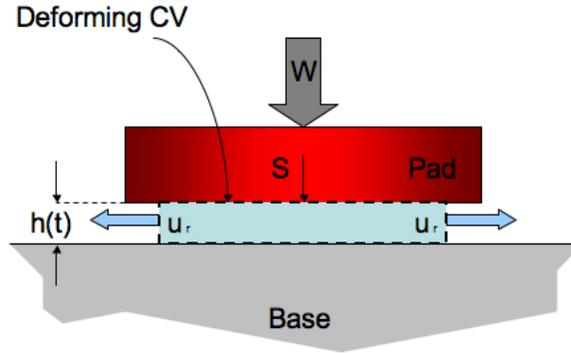
$$\frac{\partial}{\partial t} \int_{CV} \rho dV + \int_{CV} \rho (\underline{V} - \underline{V}_{cs}) \cdot \underline{n} dA = 0, \quad (6.21n)$$
