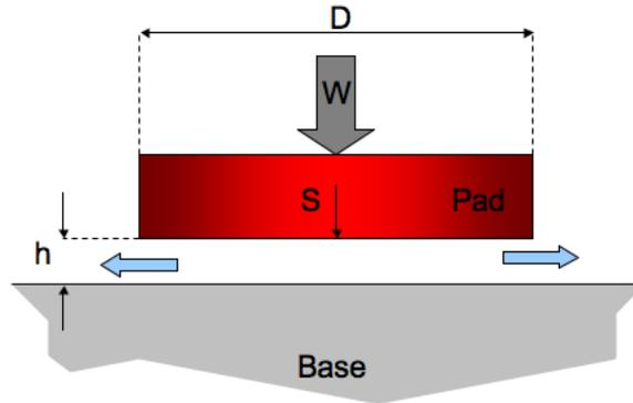
The sketch shows a circular bearing pad which rests on a flat base through the intermediary of a film of viscous liquid of instantaneous thickness  $h(t)$ . The load  $W$  causes the pad to sink slowly at the speed  $S$ , and this squeezes the liquid out from under the pad. Assume that  $h \ll D$ , that the viscosity is very high, and that the speed  $S$  is very small.
