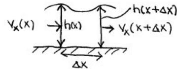
$$\Rightarrow \left[ \frac{\partial h}{\partial t} + \frac{\partial}{\partial x} \left( \int_0^h v_x dy \right) = \frac{\partial h}{\partial t} + \frac{\partial Q}{\partial x} = 0 \right] \quad (3)$$
