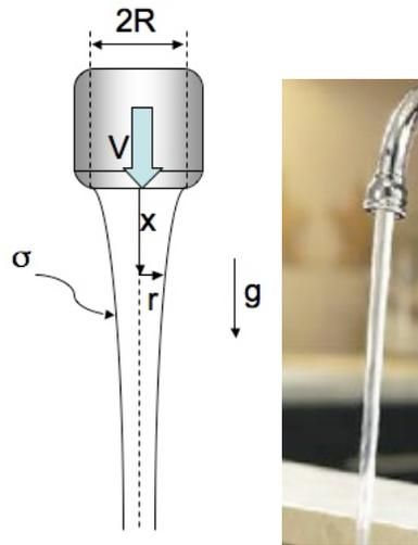
An incompressible, inviscid liquid flows with speed  $V$  vertically downward from the nozzle of the radius  $R$ . The liquid density  $\rho$  is high compared with that of the ambient air. The surface tension between the liquid and the air is  $\sigma$ .
