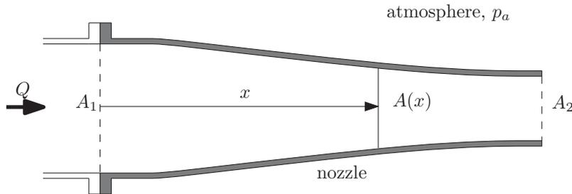
A nozzle with exit area  $A_2$  is mounted at the end of a pipe of area  $A_1$ , as shown. The nozzle converges gradually, and we assume that the flow in it is (i) approximately uniform over any particular station  $x$ , (ii) incompressible, and (iii) inviscid. Gravitational effects are, furthermore, taken as negligible. The volume flow rate in the nozzle is given as  $Q$  and the ambient pressure is  $p_a$ .
