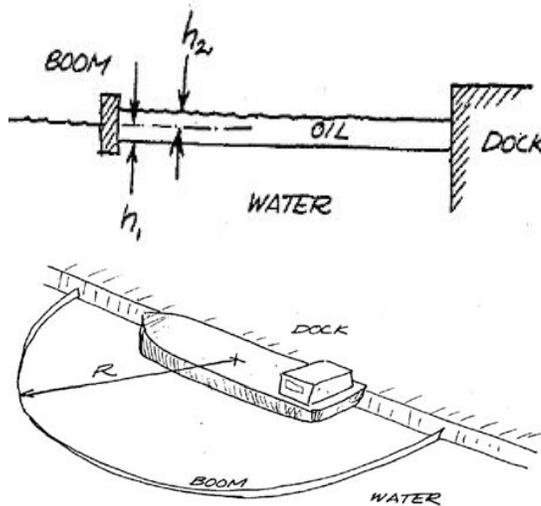
Oil Spills may occur in ports where oil tankers are loaded. The density of oil,  $\rho$  is less than that of water  $\rho_w$ , and the two fluids are immiscible, so that when a spill occurs the oil simply spreads out in a layer on top of the water. To contain any possible spills, a semi-circular “oil boom” is deployed at a radius  $R$  around the dock where the loading takes place.
