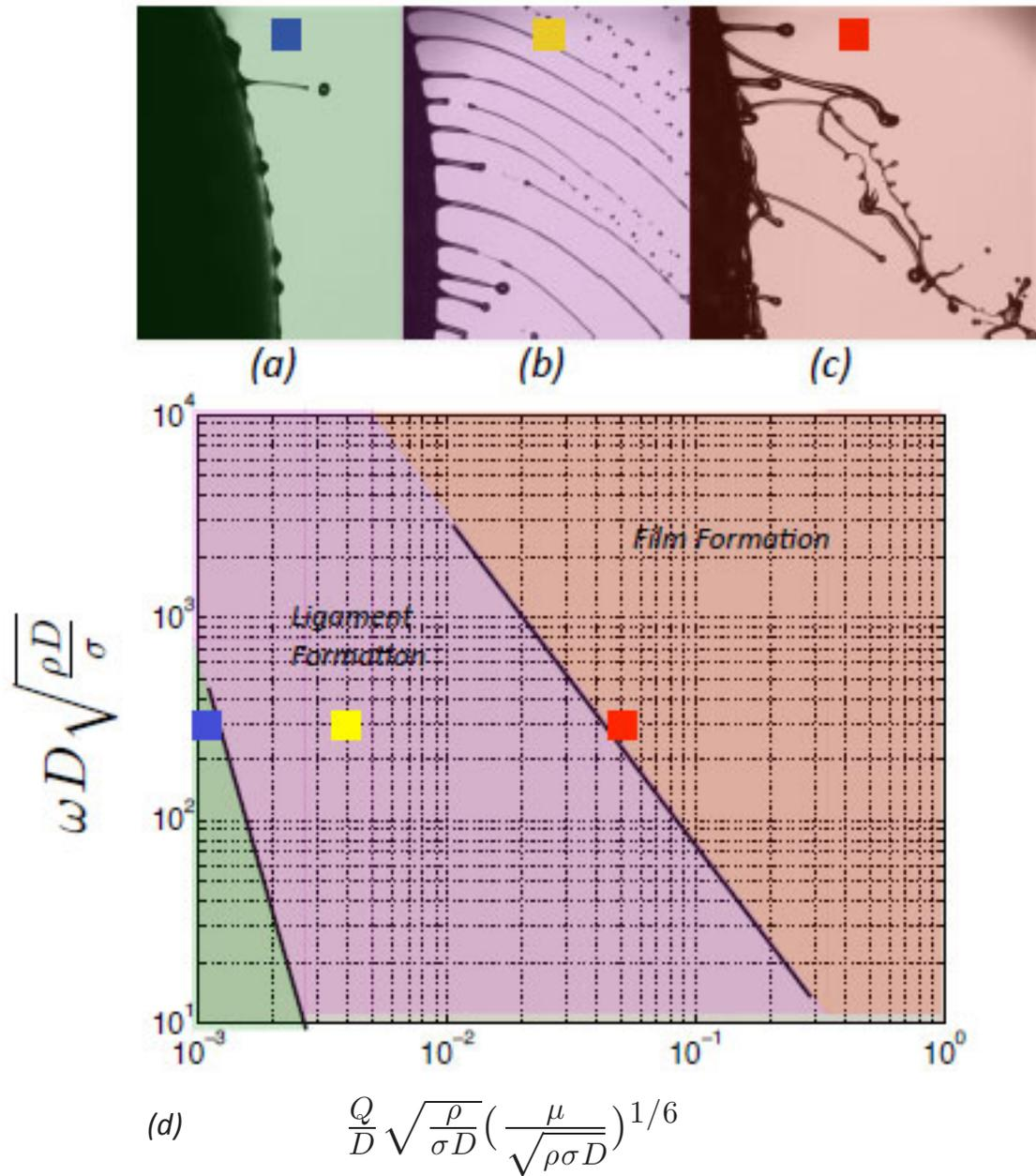
Figure 5: (a) Single drop formation stage (b) Ligament formation stage (c) Liquid film formation stage. (d) Results from Hinze et al. ([1]) showing the performance map for the rotary atomization described with dimensionless groups introduced in this problem.
