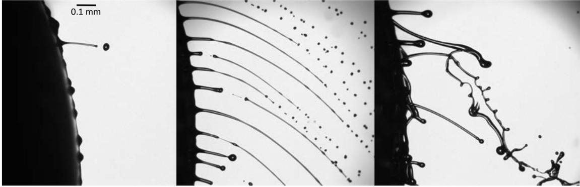
Figure 1: Rotary atomization at different flow rates (Image: Bavand-HML).
