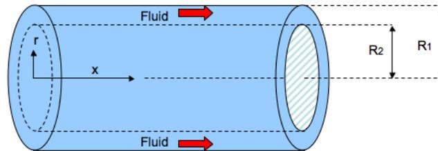
Consider a steady, fully developed laminar flow in an annulus with inside radius  $R_2$  and outside radius  $R_1$ .
