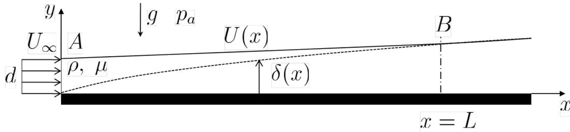
Momentum flows in the  $x$ -direction through planes  $A$  and  $B$  and through the  $y = 0$  plane via shear stresses acting on the plate. No shear stresses contribute to the  $x$ -component of the momentum flux on plane  $B$ . No momentum is flowing through the free surface.
