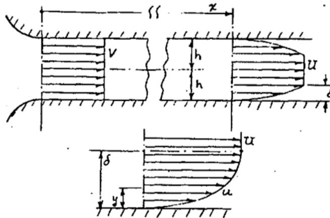
Consider the two-dimensional, incompressible, steady flow of a fluid of constant viscosity in the entrance region of a slit of width  $2h$ . The flow enters the tube ( $x = 0$ ) with the uniform velocity  $V$ . At distance  $x$  from the entrance, the boundary layer thickness is  $\delta$ , and the core flow has the speed  $U$ . The boundary layer is laminar.
