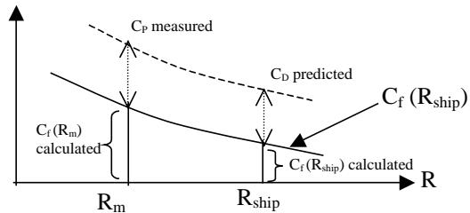
**Caution:** In an experiment, the boundary layer must be in the same regime (i.e., turbulent) as the prototype. Therefore turbulence stimulator(s) must be added.
