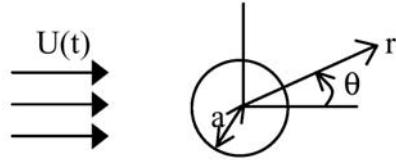
$$\phi(r, \theta, t) = U(t) \left( r + \underbrace{\frac{a^3}{2r^2}}_{\text{dipole for sphere}} \right) \cos \theta$$
