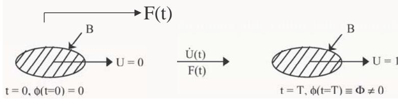
where we define  $\Phi$  to denote the velocity potential that corresponds to unit velocity  $U = 1$ . In this case the velocity potential  $\phi$  for an arbitrary velocity  $U$  is  $\phi = U\Phi$ .
