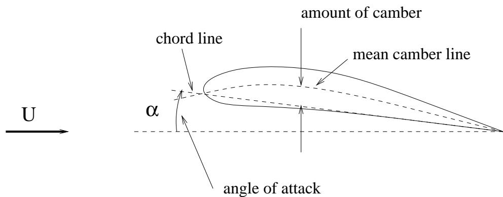
Lift  $\perp$  to  $\vec{U}$  and Drag  $\parallel$  to  $\vec{U}$
