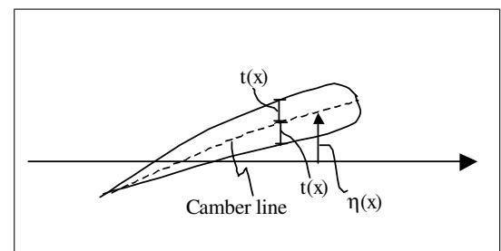
For linearized theory, i.e. thin wing at small AoA, the lift on the wing depends only on the camber line **but not** on the wing thickness. Therefore, for the following analysis we approximate the wing by the camber line only and ignore the wing thickness.
