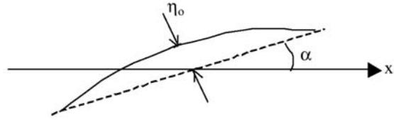
$$C_L = C_{L\alpha} + C_{L\eta} = 2\pi\alpha + 4\pi\frac{\eta_0}{\ell}$$
