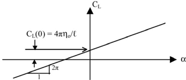
Lift coefficient  $C_L$  as a function of the angle of attack  $\alpha$  and  $\frac{\eta_0}{\ell}$ .
