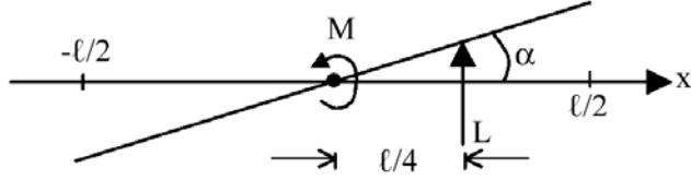
Linear lifting theory gives  $\gamma(x)$ , which can be integrated to give the lift coefficient  $C_L$ ,
