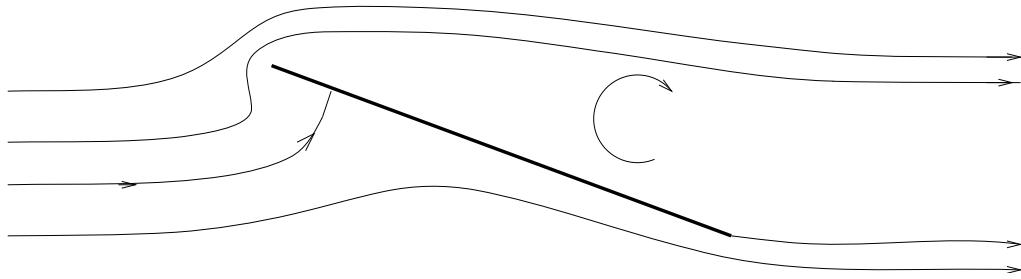
Excessive angle of attack leads to separation at the leading edge.
