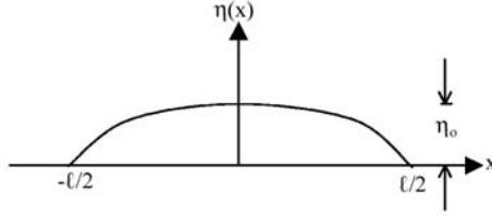
Linear lifting theory gives  $\gamma(x)$ , which can be integrated to give the lift coefficient  $C_L$ ,
