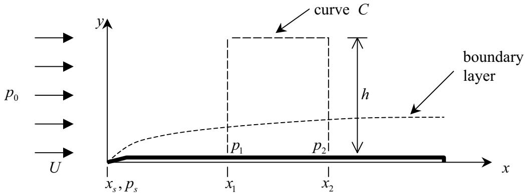
The point  $x_s$  at the leading edge of the plate is a stagnation point where the stagnation pressure is  $p_s$ . The pressure at point  $x_1$  is  $p_1$ . Point  $x_2$  is assumed to be far enough downstream in the boundary layer that  $p_2$  equals the free stream pressure  $p_0$ .
