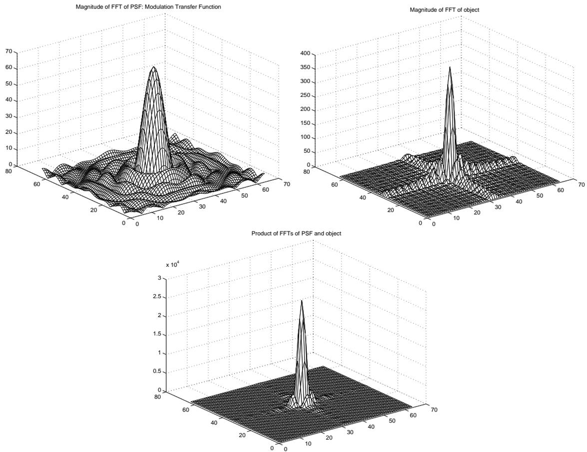
Figure 6: Frequency domain based convolution: the magnitude of the Fourier transforms of (a) the point-spread function, (b) the object, and (c) the resulting image.
