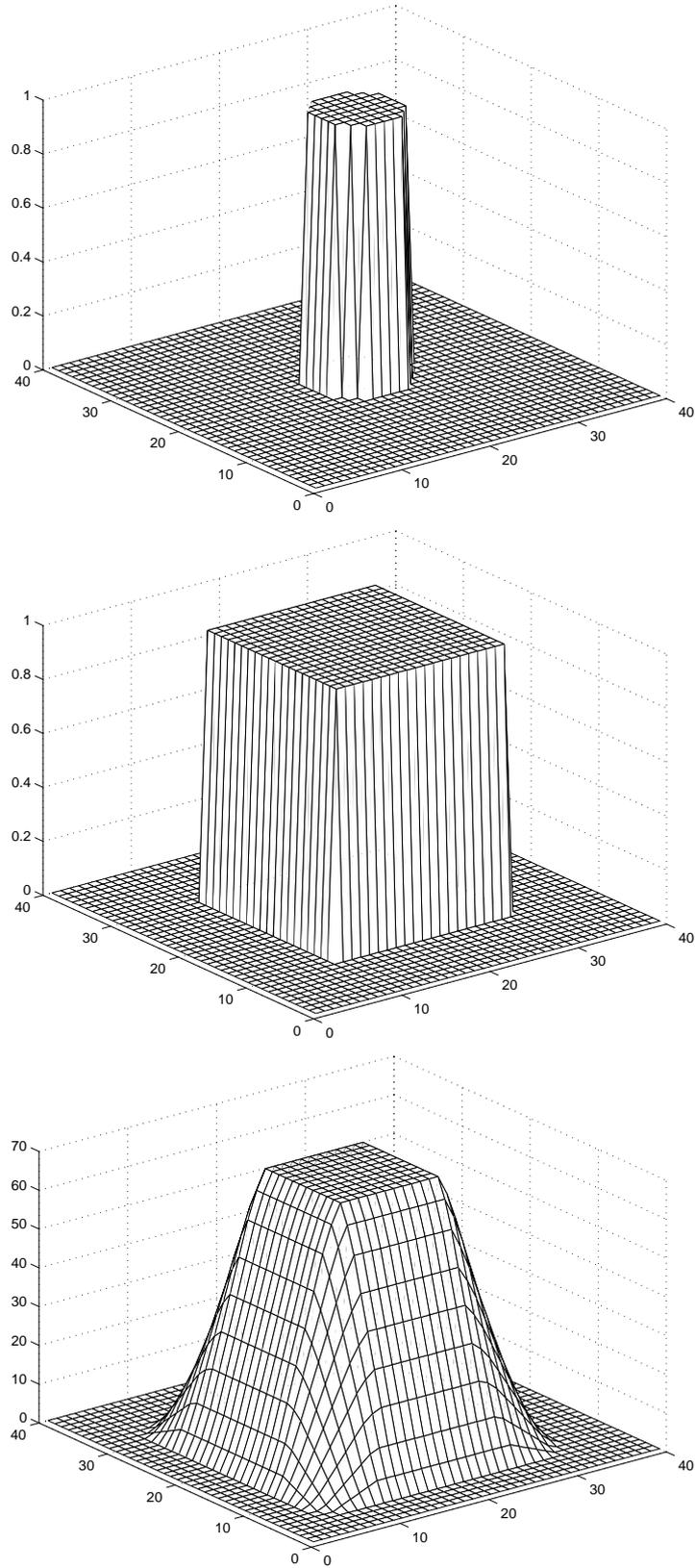
Figure 2: Two-dimensional convolution: (a) A circular point-spread function, ( $r = 5$ ), (b) a uniform rectangular  $20 \times 20$  object, and (c) the image formed by convolution.
