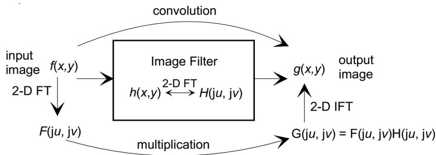
Figure 4: Two dimensional image filtering.
