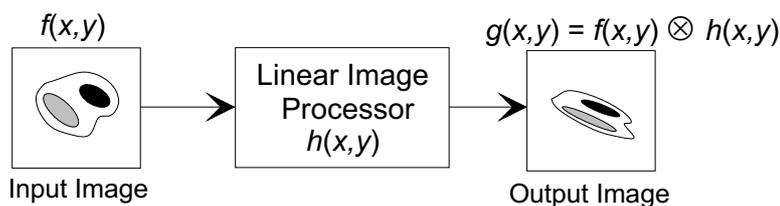
Figure 1: A two-dimensional linear image processing system.
