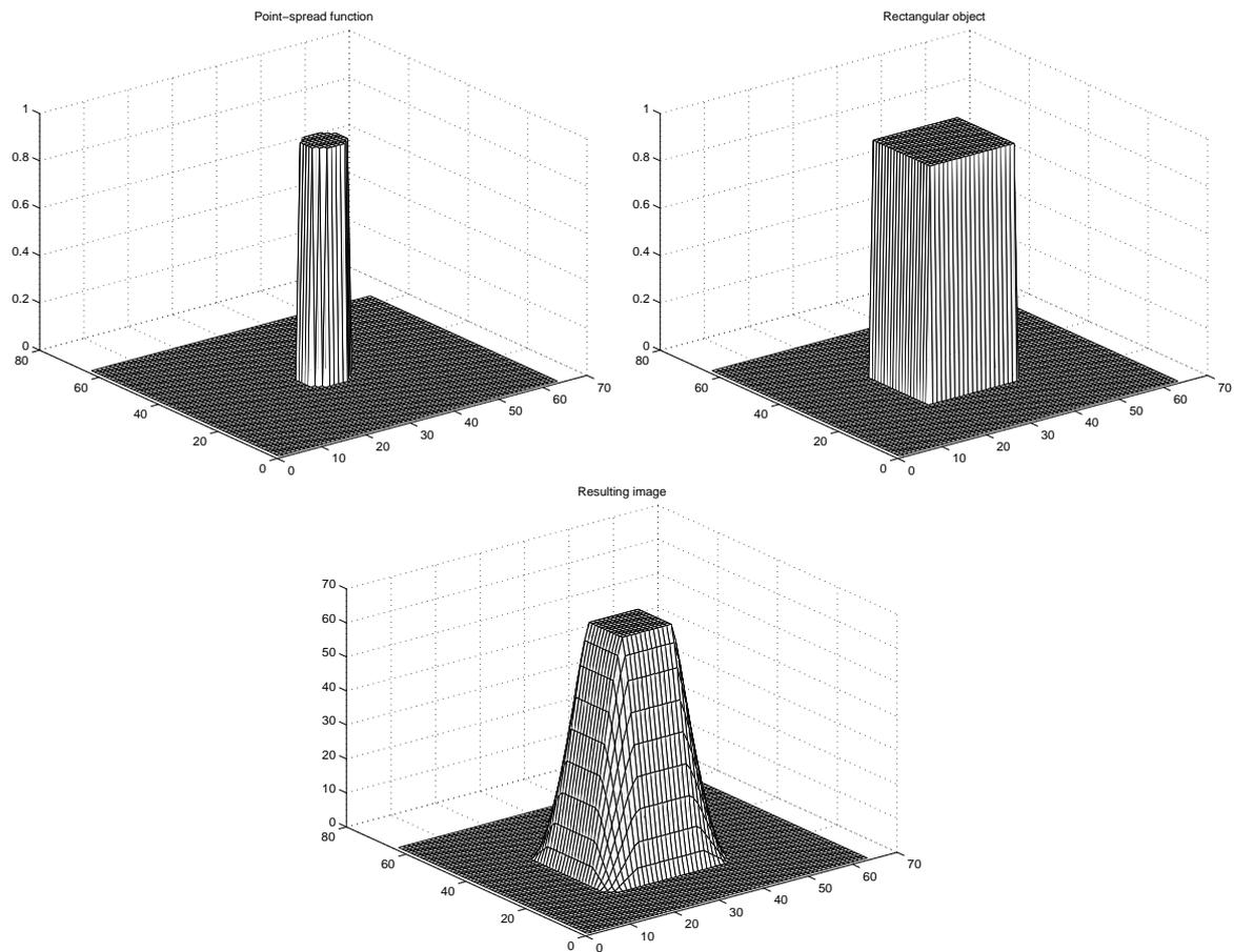
Figure 5: Frequency domain based convolution:(a) the point-spread function, (b) the object, and (c) the resulting image.
