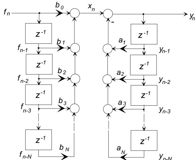
The following MATLAB code implements the Direct Form I structure in a point-by-point filtering function.
