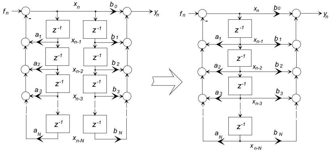
Notice that only a single delay register is required for the Direct Form II structure, as is shown on the right.
