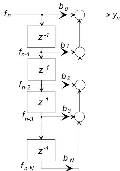
The following MATLAB code implements this structure in a point-by-point filtering function:
