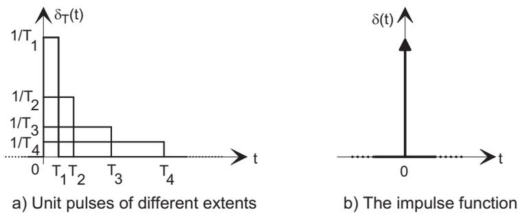
Figure 1: Unit pulses and the Dirac delta function.
