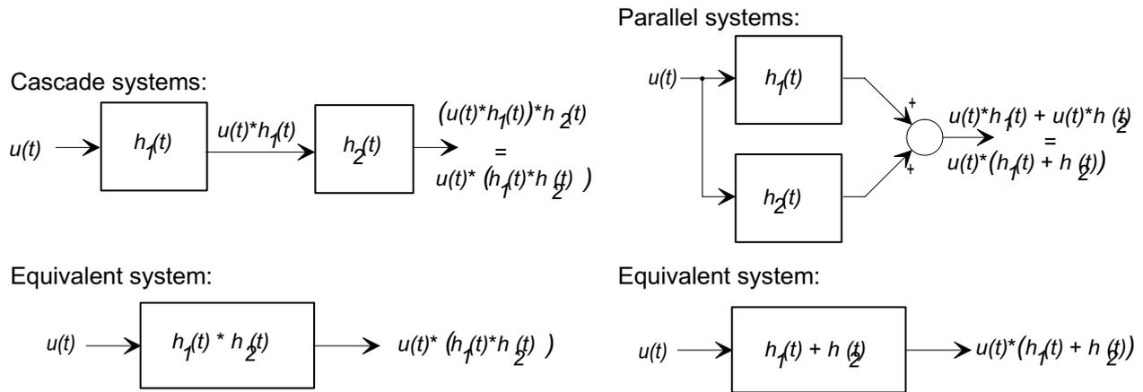
Figure 7: Impulse response of series and parallel connected systems.
