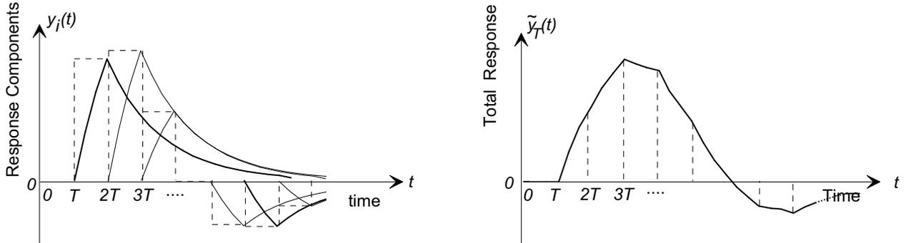
Figure 4: System response to individual pulses in the staircase approximation to  $u(t)$ .
