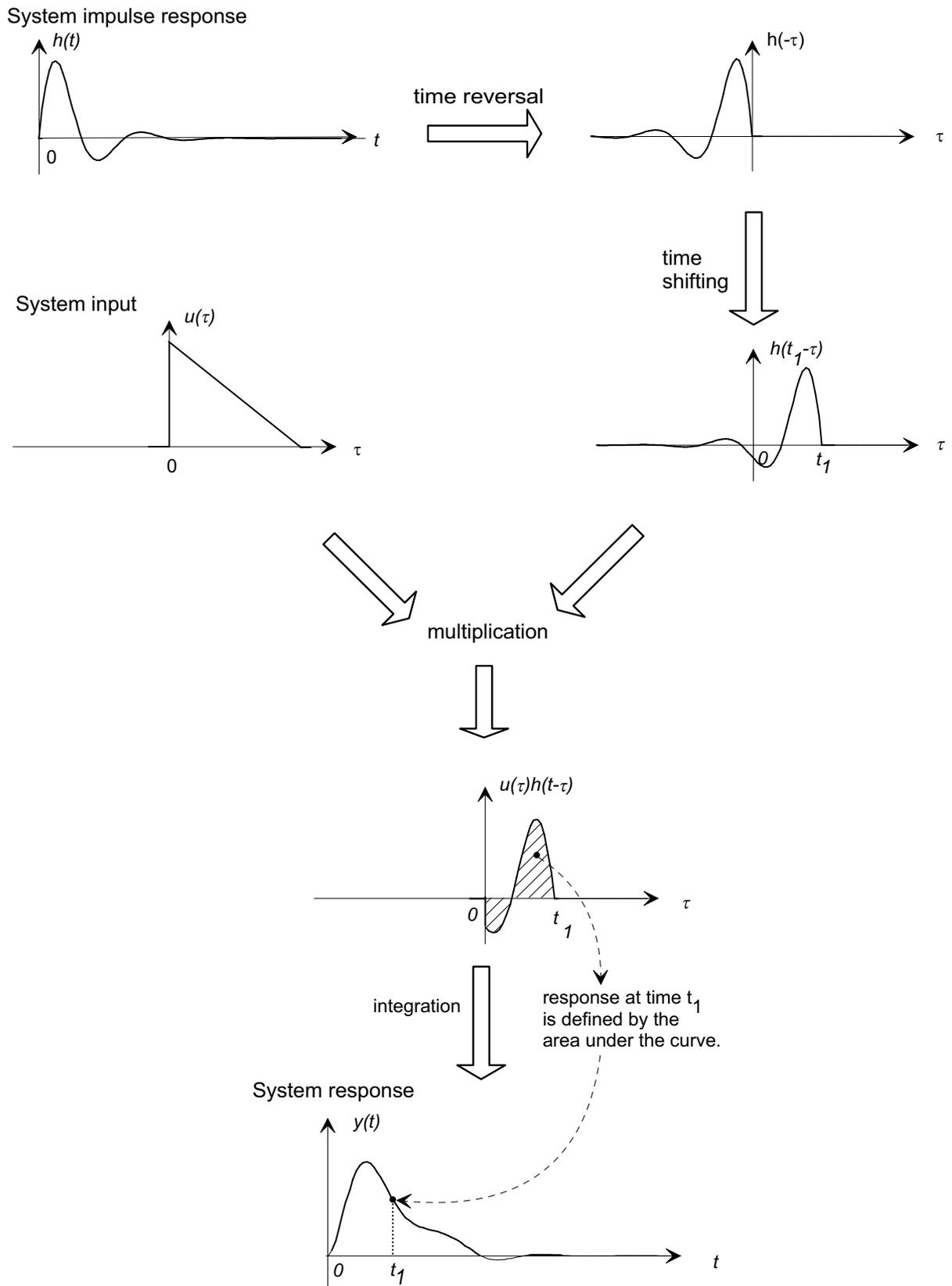
Figure 5: Graphical demonstration of the convolution integral.
