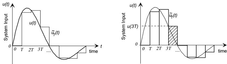
Figure 2: Staircase approximation to a continuous input function  $u(t)$ .
