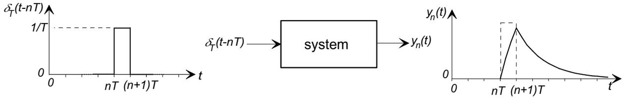
Figure 3: System response to a unit pulse of duration  $T$ .
