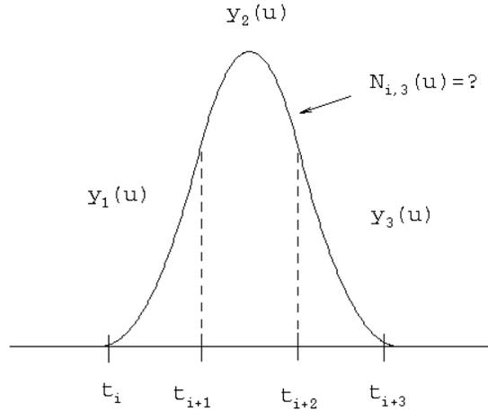
Figure 6.2: Plot of 3<sup>rd</sup> order B-spline basis function.
