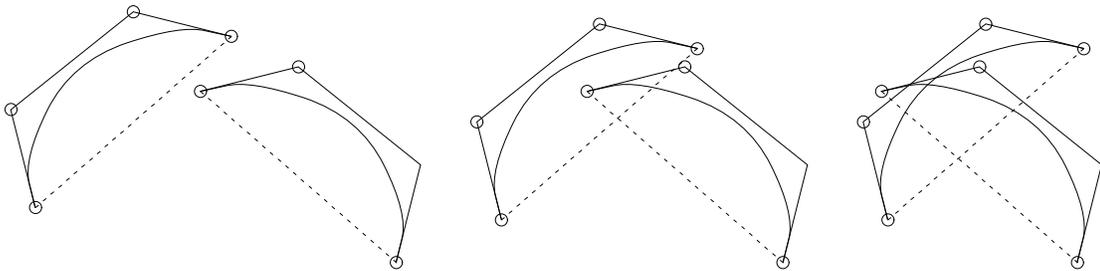
Figure 4.17: Comparison of convex hulls of Bézier curves as a means to detect intersection
