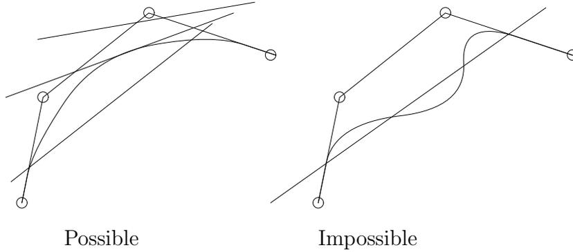
Figure 4.18: Variation diminishing property of a cubic Bézier curve
