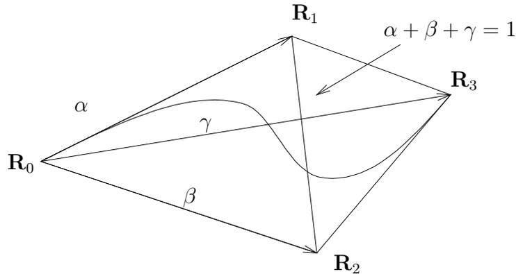
Figure 4.15: Convex hull of a 3D space cubic Bézier curve is a tetrahedron.
