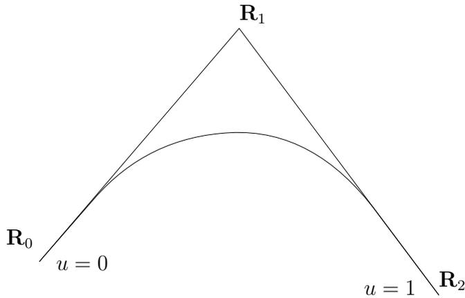
Figure 4.7: Illustration of end conditions for a quadratic Bézier curve.
