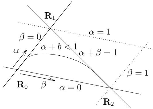
Figure 4.14: Convex hull of a quadratic Bézier curve.
