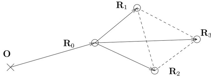
Figure 4.12: Geometry of Bézier curves is invariant under translation.
