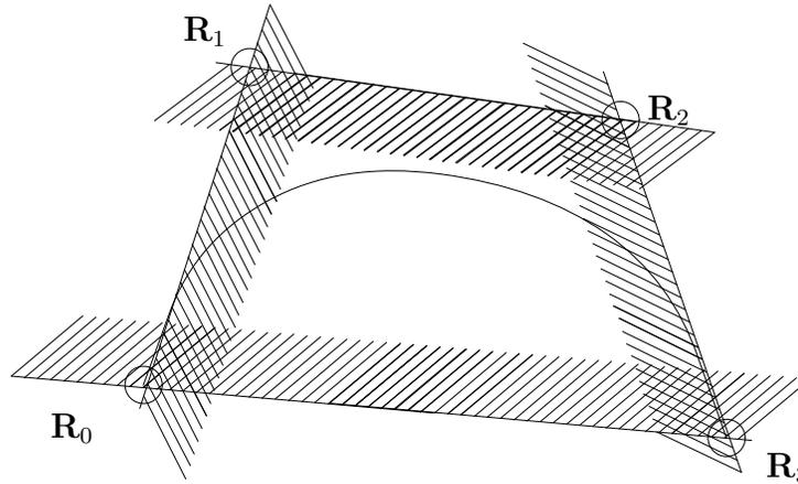
Figure 4.16: Convex hull of a planar cubic Bézier curve
