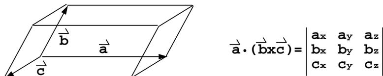
Figure 2.11: The computation of the volume of a parallelepiped
