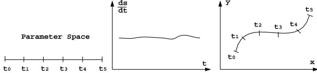
Figure 2.6: When parametric speed does not vary, parameter values are uniformly spaced along a parametric curve.
