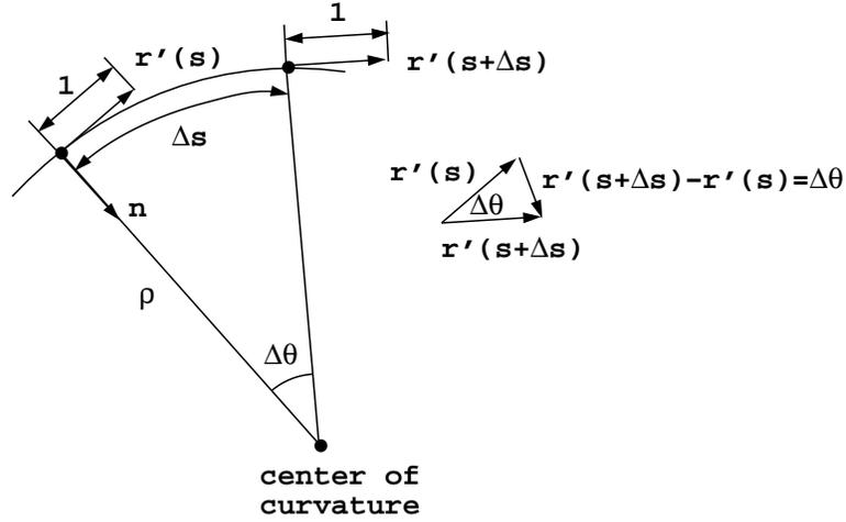
Figure 2.8: Derivation of the normal vector of a curve.
