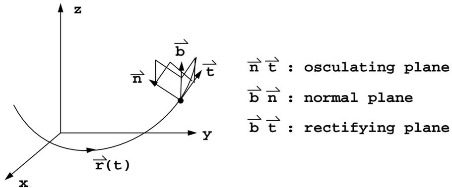
Figure 2.10: The tangent, normal, and binormal vectors define an orthogonal coordinate system along a space curve.
