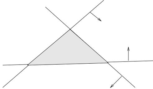
Figure 1.20: Half space technique of model representation.
