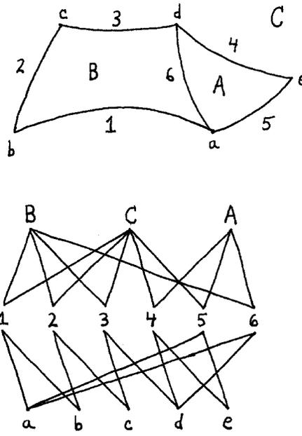
Figure 1.16: Cell data structure.
