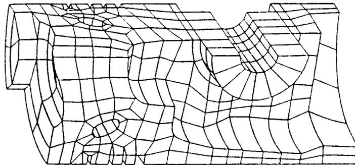
Figure 1.15: A cell decomposition (finite element mesh).
