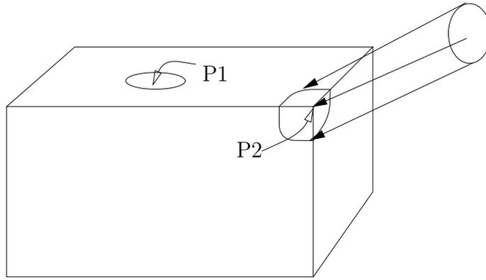
Figure 1.5: The cube is a two manifold object.
