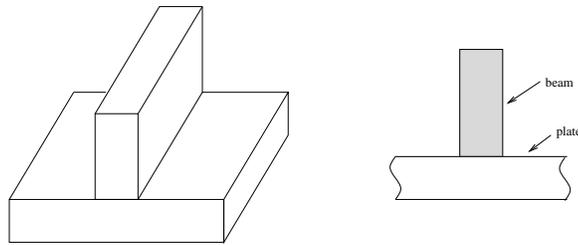
Figure 1.7: Beam welded to a plate.
