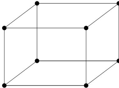
Figure 1.1: Wire frame model of a cube.
