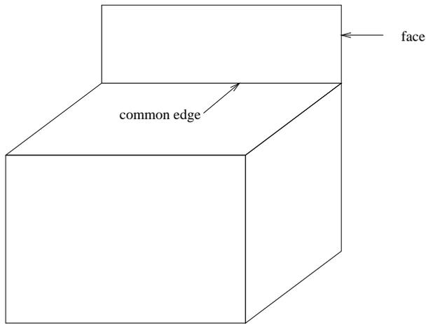
Figure 1.6: Examples of non-two manifold models.
