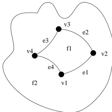
Figure 1.21: Boundary based representation Using Euler operations.
