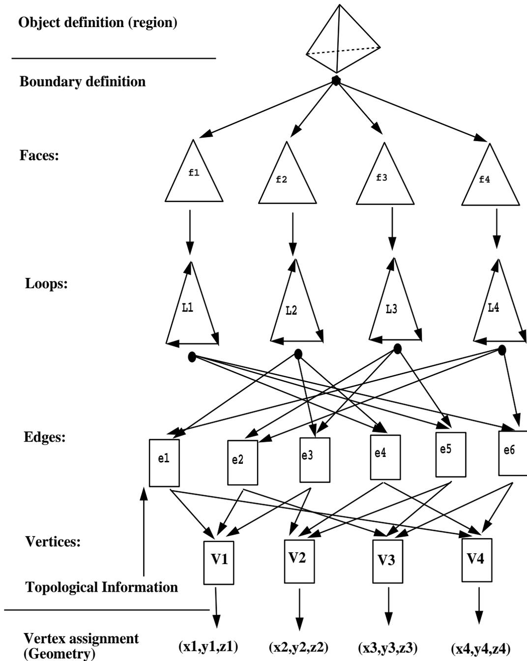
Figure 1.19: Boundary representation model for a tetrahedron
