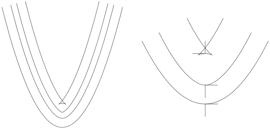
Figure 13.7: Offsets to a parabola  $\mathbf{r} = [t, t^2]$  (thick solid line) with offsets  $d = -0.3, -0.5, -0.8$ , adapted from [5]. At  $d = -0.3$  the tangent and normal vectors of the offset have the same sense that of the progenitor, while at  $d = -0.8$  they flip directions.
