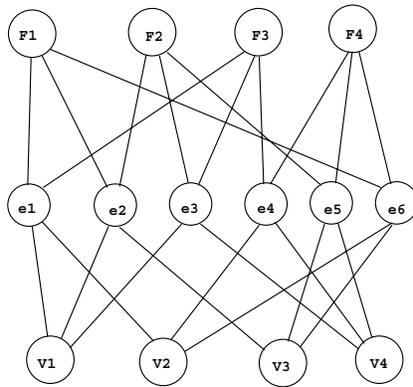
**Problem 2.** Can this incidence graph be a valid two-manifold solid's boundary? If yes, sketch a 3-D figure satisfying the incidence graph, otherwise explain. Below,  $F_i$  are planar faces,  $e_j$  are edges, and  $V_k$  are vertices.
