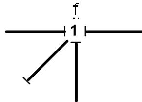
Figure 3.32: Example of a permissible causal assignment for a one junction.
