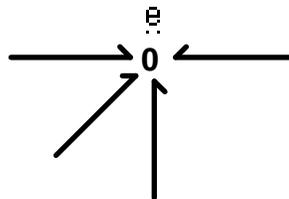
Figure 3.27: Sign convention assumed in flow continuity equation 3.27.
