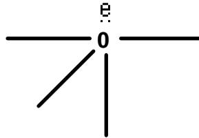
Figure 3.26: Bond graph symbol for a common effort or type zero junction.
