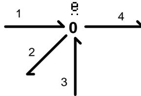
Figure 3.28: Sign convention assumed in flow continuity equation 3.28.
