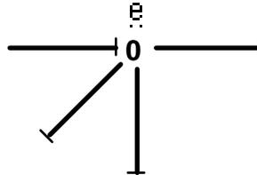
Figure 3.29: Example of a permissible causal assignment for a zero junction.
