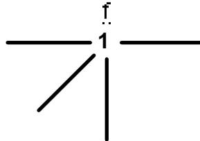
Figure 3.30: Bond graph symbol for a common flow or type zero junction.
