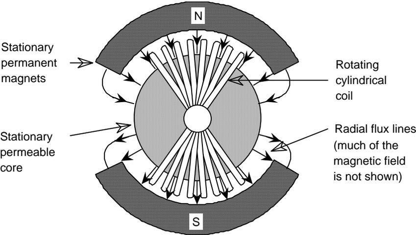
Figure 3: Schematic end-view of a D'Arsonval galvanometer modified to reduce the angle-dependence of the transduction equations.
