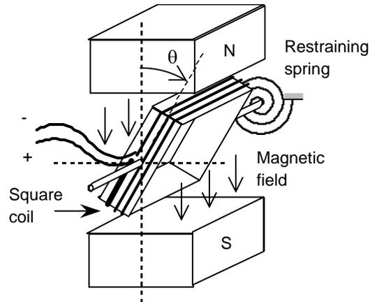
Figure 2: Sketch of a D'Arsonval galvanometer.
