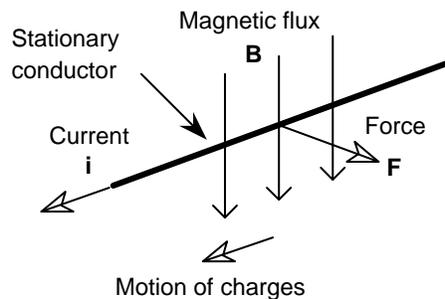
An electric field is oriented parallel to the wire. As charges move along the wire, the magnetic field makes them try to move sideways, exerting a force on the wire. The lateral force due to all the charge in the wire is:
