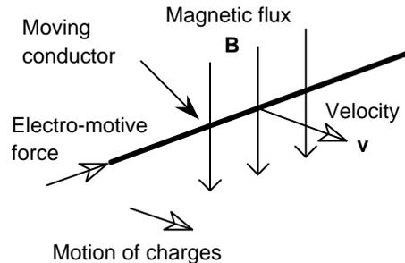
A component of charge motion is the same as the wire motion. The magnetic field makes charges try to move along the length of the wire from left to right. The resulting *electromotive force* (emf) opposes the current and is known as back-emf.
