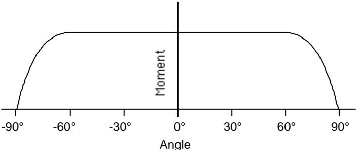
Figure 4: Sketch of half of the constant-current torque/angle relation resulting from the design of figure 3.
