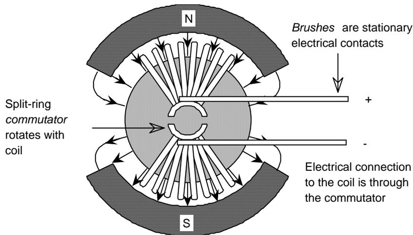
Figure 5: Schematic of the mechanical commutation system used in a direct-current permanent magnet motor.
