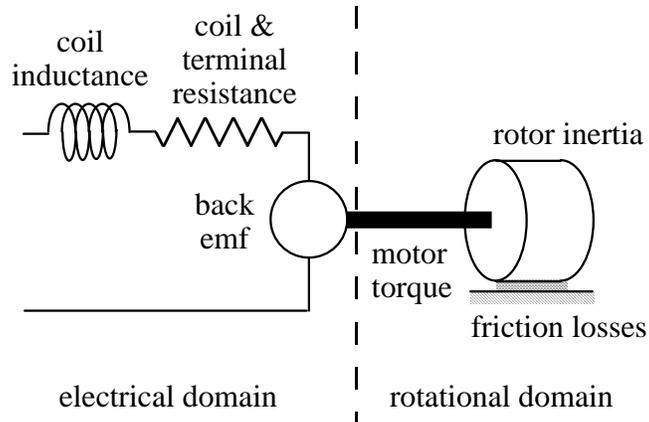
Schematic diagram of DCPMM model with “parasitic” dynamics
