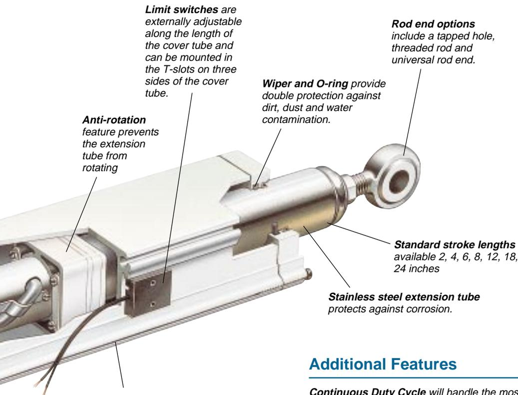
**Cover tube** of anodized extruded aluminum resists corrosion, is lightweight and allows positioning of sensors along its length.
