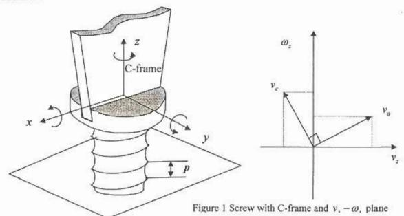
a).  $V_{\Xi}$  and  $W_{\Xi}$  are related:  $V_{\Xi} = \frac{P}{2\pi}W_{\Xi}$ , or  $V_{\Xi}$ :  $W_{\Xi} = P:2\pi$ . This means that in the  $V_{\Xi} - W_{\Xi}$  plane the direction of admissible motion, denoted by vector Q is  $Q = \begin{bmatrix} P \\ 2\pi \end{bmatrix}$
