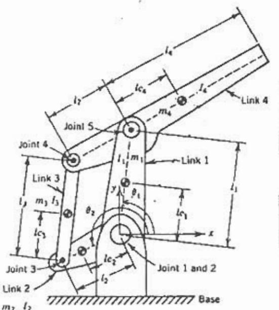
Figure 1 Planar robot with parallelogram mechanism
