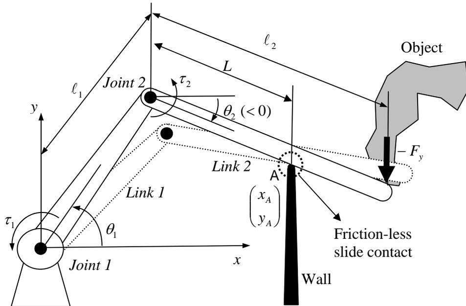
Figure 3 Rescue robot moving a heavy object
