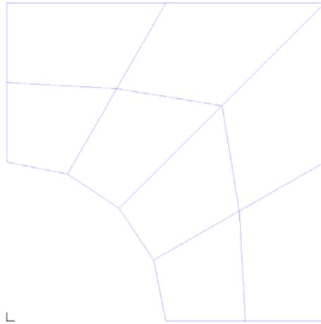
Use as the exact strain energy **E= 0.8019875218E+00** which is obtained using 20,000 9-node u/p elements.
