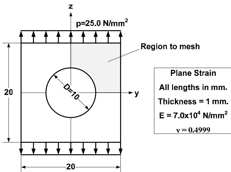
(Case 1) Use the displacement-based 4-node and 9-node elements and establish convergence curves for these elements. Thus establish the rates of convergence.
