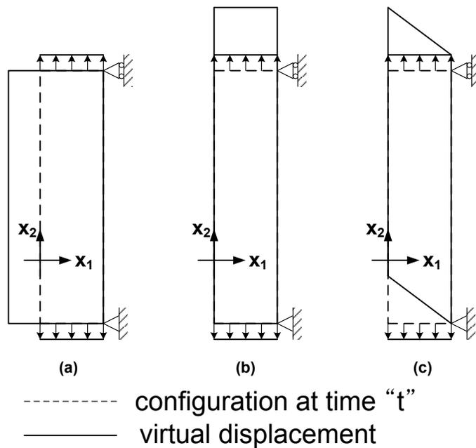
Figure 1. Three simple independent virtual displacement patterns.
