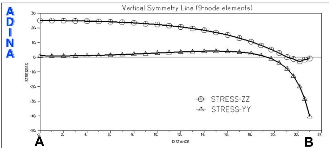
Figure 6. Stresses on the vertical symmetry line solved using 9-node elements
