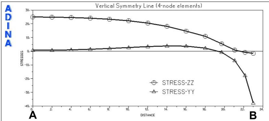
Figure 5. Stresses on the vertical symmetry line solved using 4-node elements
