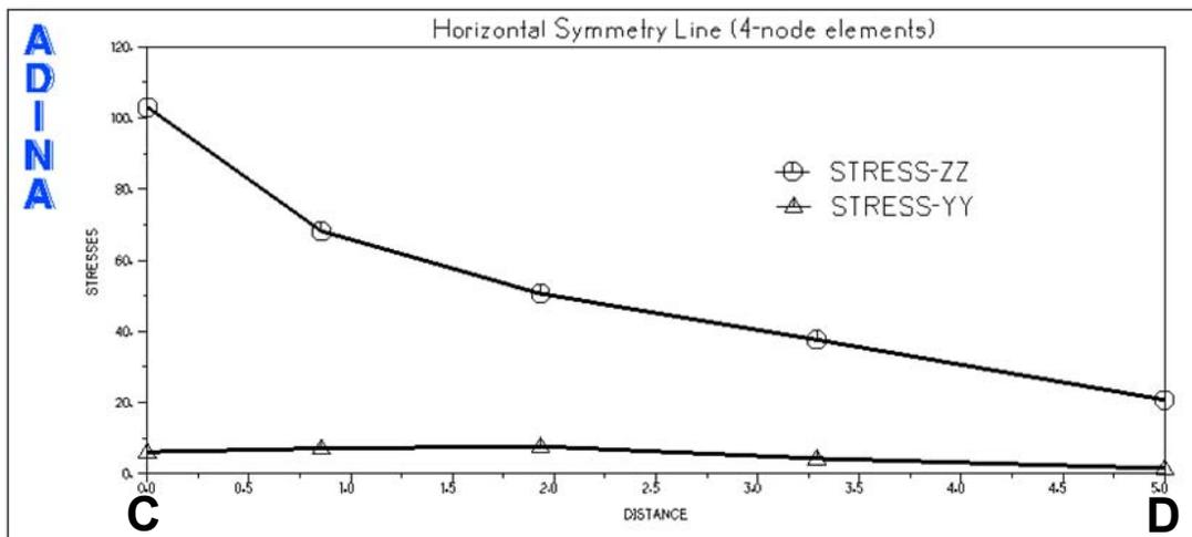
**Figure 3. Stresses on the horizontal symmetry line solved using 4-node elements**
