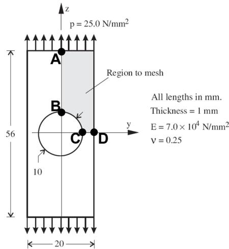
**Figure 2. Plate with a hole in tension**
