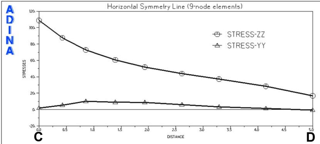
Figure 4. Stresses on the horizontal symmetry line solved using 9-node elements
