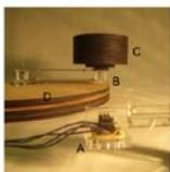
Figure 2: Experimental setup for friction measurement. Force transducer (A) is connected to contact arm (B) by a thin wire. Normal force is exerted on the contact arm by lead stack (C). Tangential force is applied using turntable (D) via the friction between the turntable surface and the contact area. Apparatus and photograph courtesy of James Peon.
