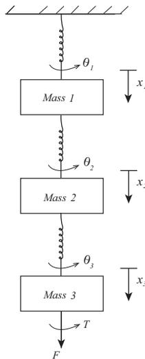
Figure 1: A triple pendulum made of 3 Wilberforce springs that is the subject of Question 4.
