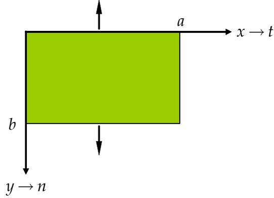
**Boundary Conditions** For edges parallel to  $x$ -axis, the normal direction is the  $y$ direction.
