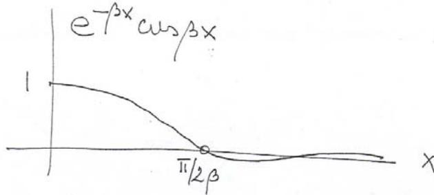
It can be conducted that the curvature and bending is confined to a narrow boundary zone of the width  $x_b = \pi/(2\beta)$ . The remainder of the shell undergoes a uniform radial contraction:
