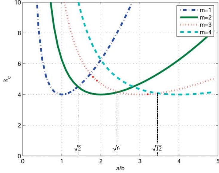
For a given  $a/b$ ,  $m$  may be chosen to yield the smallest eigenvalue. In order to minimize  $k_c$  in Eq. (281), treating  $m$  as a continuous variable produces:
