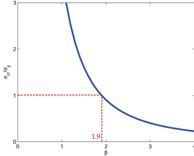
On further loading the plate beyond  $\sigma_{cr}$ , a greater proportion of the load is taken by the regions of the plate near the edge. Von Karman assumed that these edge regions, each of the width  $b_{eff}/2$ , carry the stress up to the yield while the center is stress free.
