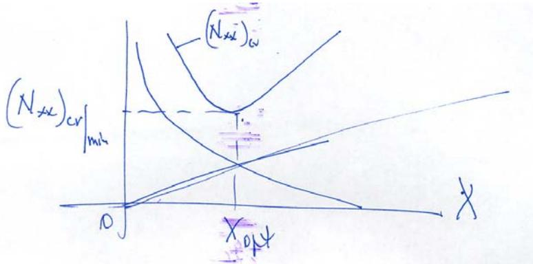
Treating  $\chi$  as a continuous variable, one can find an analytical minimum:
