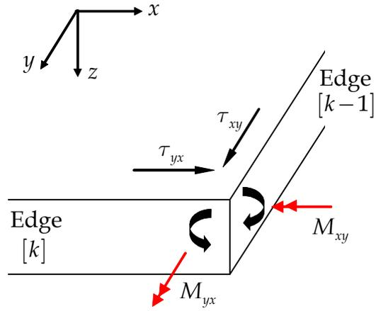
The shearing stresses produce twisting moments which are in the opposite direction:
