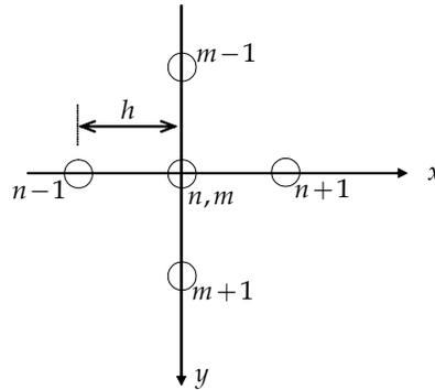
$$\begin{aligned} \left. \frac{dz}{dx} \right|_n^{backward} &\simeq \frac{z_n - z_{n-1}}{h} \\ \left. \frac{dz}{dx} \right|_{n+1}^{forward} &\simeq \frac{z_{n+1} - z_n}{h} \end{aligned} \quad (215)$$
