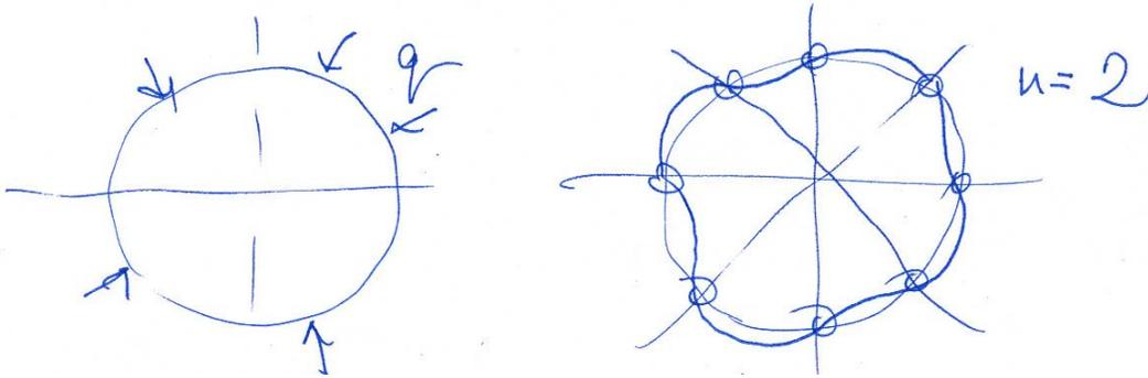
The solution of centrally directed pressure loading case is:
