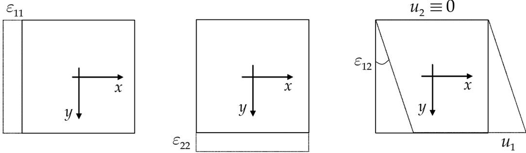
Therefore,  $\varepsilon_{11}$  and  $\varepsilon_{22}$  are the tensile strain in the two directions, and  $\varepsilon_{12}$  is the change of angles, i.e. shear strain.
