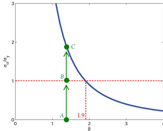
**Stowell's Theory for the Buckling Strain** Stowell developed the theory of plastic buckling for simply-supported square plates loaded in one direction.
