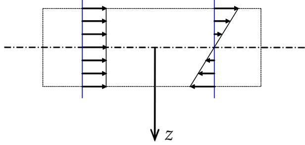
5. The out-of-plane displacement is independent of the  $z$ -coordinate, i.e.  $u_{3,3} = 0$ .
