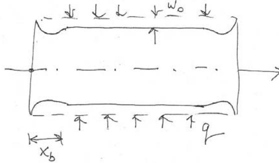
For the sake of simplicity, this localized bending can be neglected ( $D \rightarrow 0$ ). Then, from Eq. (379), the hoop membrane force is related to the lateral pressure by  $N_{\theta\theta} = qa$  and the pre-buckling solution is:
