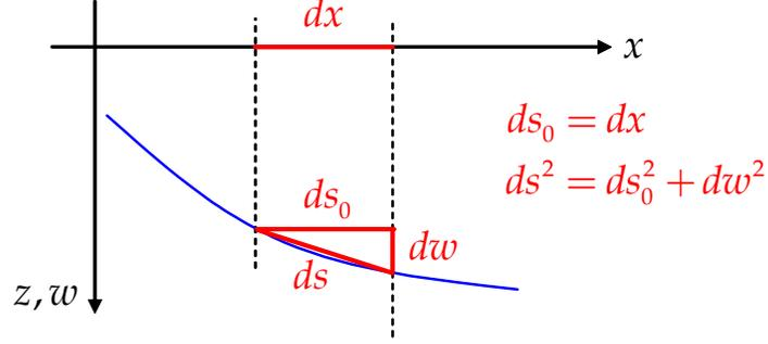
Thus, the conclusion is that the nonlinear term  $\frac{1}{2}w_{,\alpha} w_{,\beta}$  represents the change of length of the plate element due to finite rotations.
