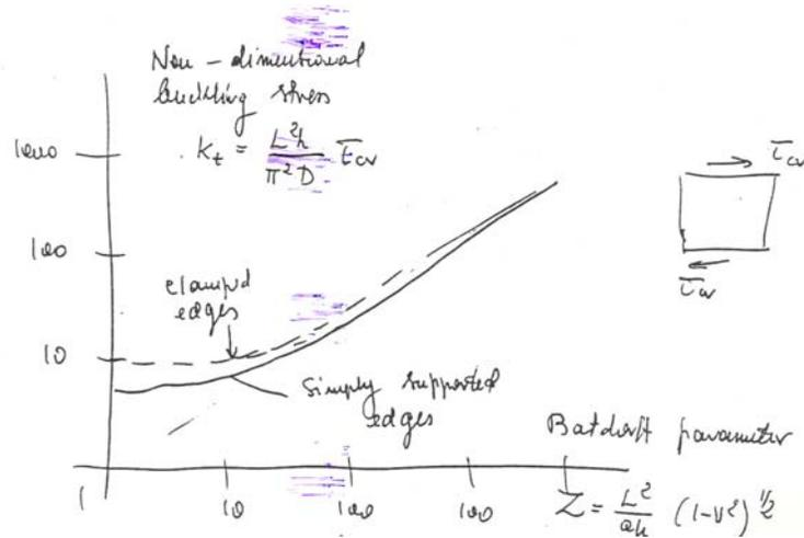
As the radius of the shell approaches infinity, the critical stress coefficient for simply supported and clamped edge approaches respectively the value 5.35 and 8.98 corresponding to plates under the shear loading.
