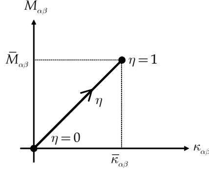
$$\begin{aligned} M_{\alpha\beta} &= \hat{M}_{\alpha\beta}(\kappa_{\alpha\beta}) \\ &= \hat{M}_{\alpha\beta}(\eta \bar{\kappa}_{\alpha\beta}) \\ &= \eta \hat{M}_{\alpha\beta}(\bar{\kappa}_{\alpha\beta}) \end{aligned} \quad (49)$$
