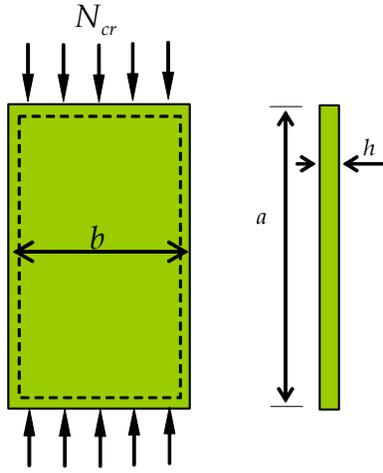
Transition from global to local buckling can be calculated by  $(P_{cr})_{column} = (P_{cr})_{plate}$ :
