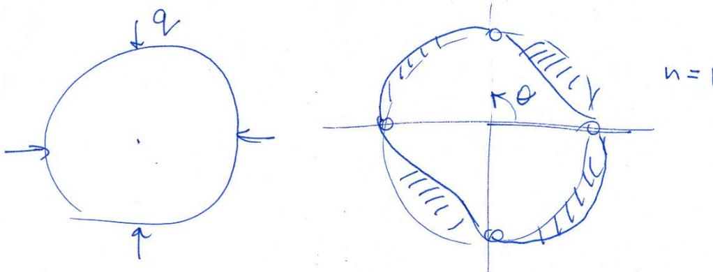
The Donnell solution should be compared with more exact solution of the ring buckling problem which take into account a more complex incremental displacement field with both  $w(\theta)$  and  $v(\theta)$ . Here, a distinction should be made between the centrally directed pressure (as in all preceding analysis) and the field -pressure loading where pressure is always directed normal to the deformed surface.
