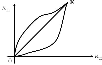
Calculate the energy density stored when the curvature reaches a given value  $\bar{\kappa}_{\alpha\beta}$ . Consider a straight loading path:
