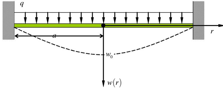
**Membrane Solution** From the symmetry and clamped boundary condition, the radial displacement  $u_r$  reads:
