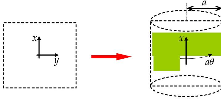
Can the strain-displacement relation for a cylinder be derived from similar relation for a flat plate?
