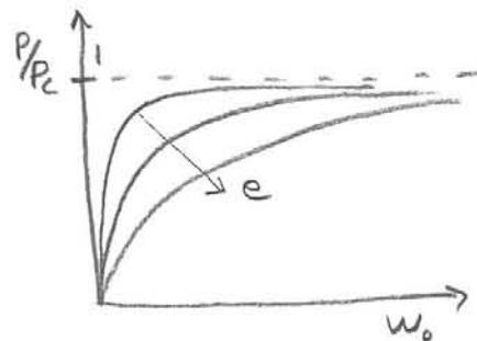
Example: Column on an elastic foundation
