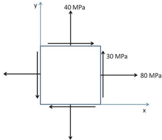
The stress state on the positive  $x$ -face is  $\sigma = +80$  MPa, and  $\tau = -30$  MPa (because of the sign convention defined above).
