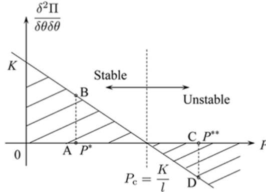
Figure 9.2: Stable and unstable range in column buckling.
