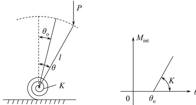
Figure 9.7: The initial inclination angle  $\theta_o$  is a measure of structural imperfection.
