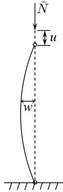
Figure 9.6: Initial and deformed elastic column.
