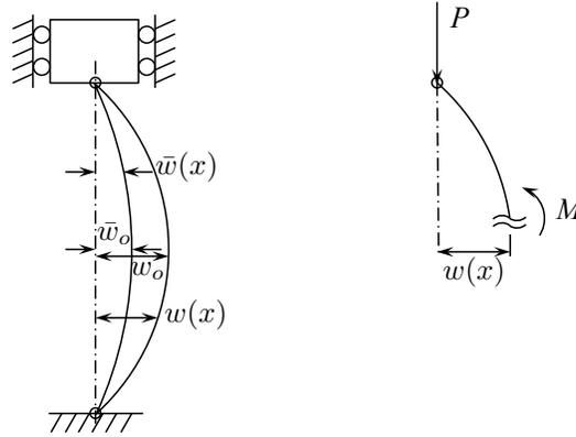
Figure 9.9: A continuous imperfect column and the free body diagram.
