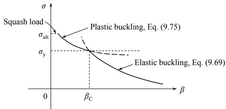
Figure 9.13: Range of elastic and plastic buckling.
