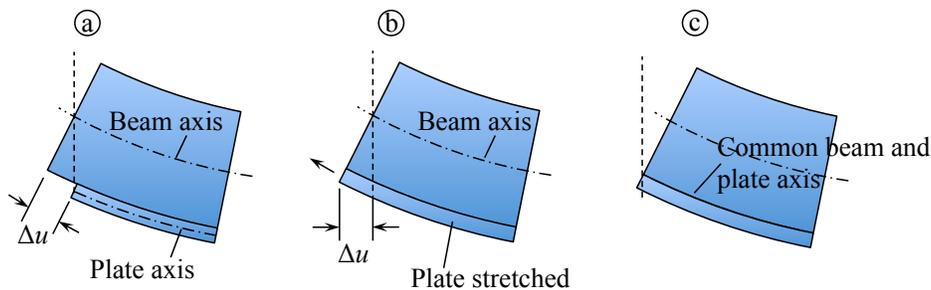
Figure 7.14: Incompatible and compatible interface between beam (stiffener) and plate.
