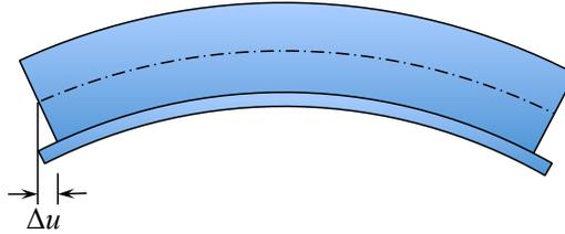
Figure 7.8: The length of the bent plate is the same as the beam axes. Relative displacement at the interface is denoted by  $\Delta u$ .
