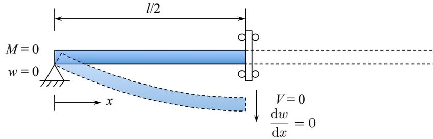
Figure 5.4: Simply-supported plate with symmetry boundary conditions.
