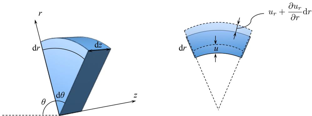
Figure 2.8: Change of length in the radial direction.
