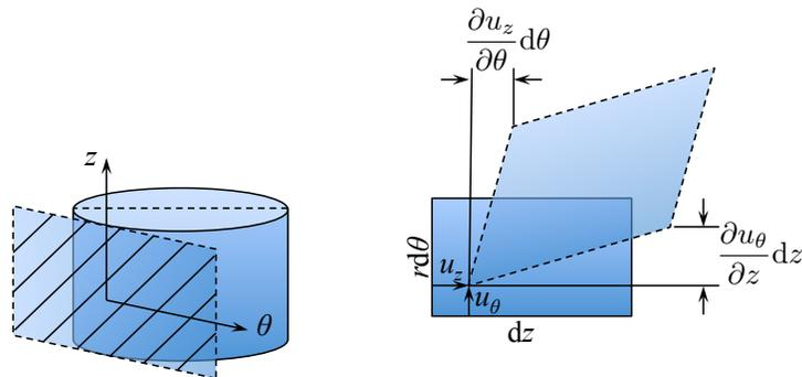
Figure 2.12: Visualization of the strain component  $\epsilon_{\theta z}$ .
