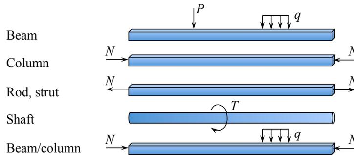
Figure 2.13: The type of loading distinguishes between *five* different types of structures.
