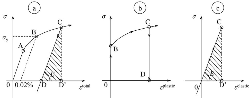
Figure 12.1: Elastic, plastic and total stress-strain curve.
