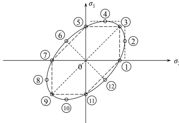
Figure 12.7: The von Mises ellipse in the principal coordinate system.
