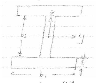
$$I_{yy} = \frac{1}{12}tb_2^3 + 2b_1t\left(\frac{b_2}{2}\right)$$
