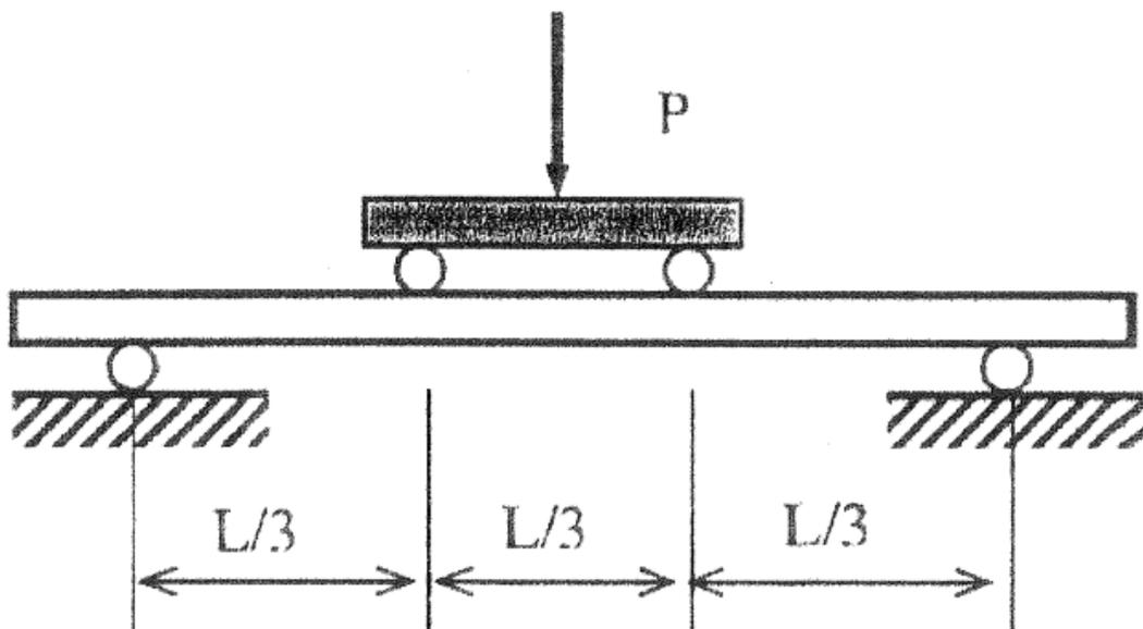
Consider the four –point bending of a beam of length  $L$ . The beam is loaded by two rollers parted by a distance of  $L/3$ . The material of the beam is rigid, perfectly plastic. Determine the load capacity of the beam under two different end conditions.
