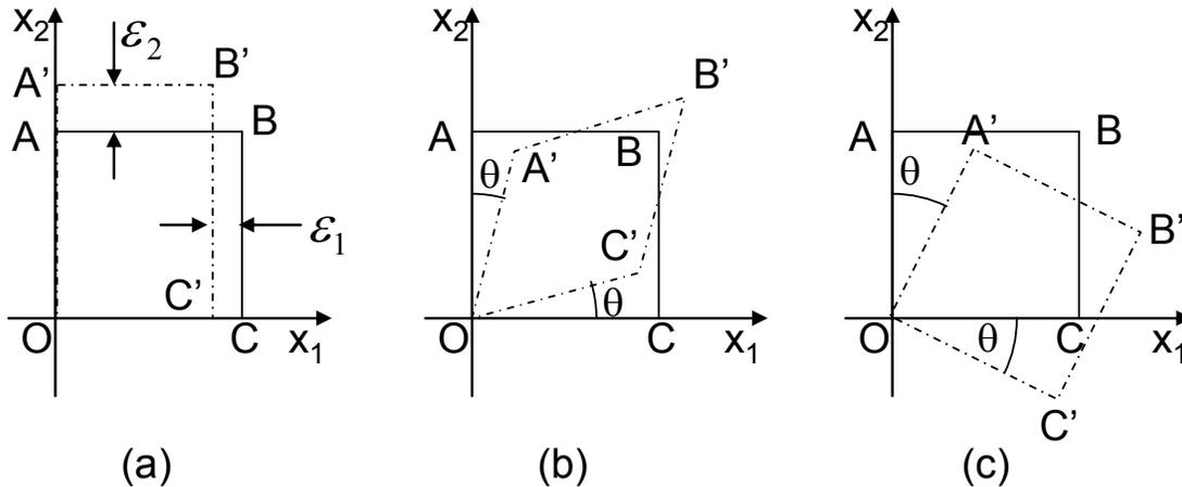
**Problem 2-4:** The strain (plane strain) in a given point of a body is described by the  $2 \times 2$  matrix below. Find components of the strain tensor  $\epsilon_{x'y'}$  in a new coordinate system rotated by the angle  $\theta$ . Consider four cases  $\theta = 45^\circ, -45^\circ, 60^\circ$  and  $-60^\circ$ .
