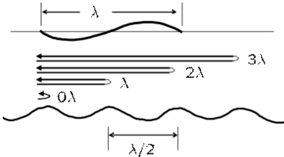
Figure 1: Bragg resonance due to constructive interference
