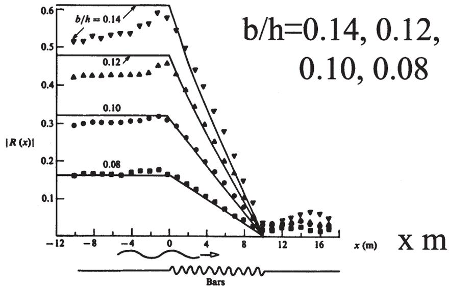
Figure 3: Bragg scattering of surface water waves by periodic bars. Comparison of theory with measurements by Heathershaw.
